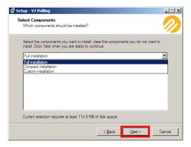
5. Select the components to install and from the drop down menu pick the type of install: Full installation, Compact installation, or Custom installation. Click **Next**.
