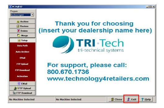
The **Exit** button (in the red box) at the bottom right of the screen closes the V7 software. The **Close** button next to it closes the current screen and returns to the main screen as above or closes the currently displayed window, but not the software.
